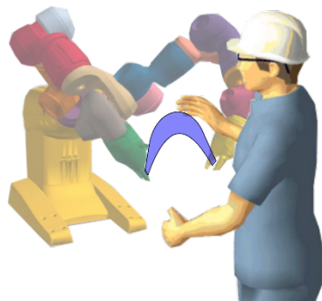
Figure : Illustration of the robotic comanipulation of a deforming object by using the collaborative robot Yumi.
